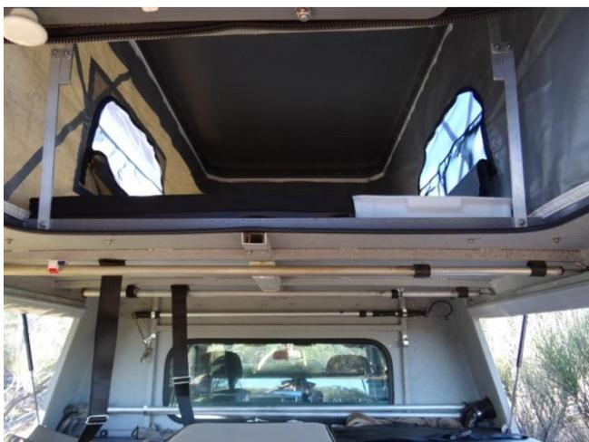
The addition of a pop-top not only solves the getting in and out of the bunk/s problem but also adds an additional bunk for one or two more persons if the top is extended forward above the cab. I say one or two extra persons because this new upper story bunk is either a very wide and comfortable single bunk or a size challenged double bunk suitable for two younger children or two
