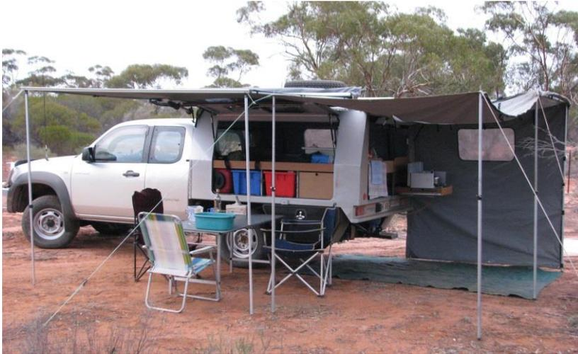
With the 4 x sideways sliding drawers shut, the Engel can be slid on its heavy duty drawer slides to the back of the vehicle for easy access. The heavy duty plastic storage containers (which can be seen in some of the pictures) are also used as drawers. The top rim of the plastic containers slides on 20mm steel tube welded under the bunks. These are
